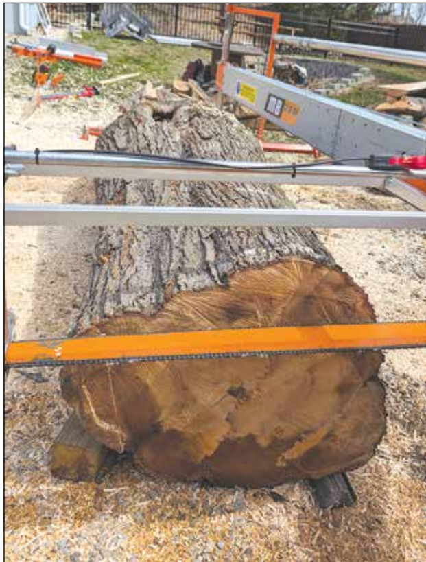
The large chainsaw attachment for the sawmill can be used to create slabs of wood up to 55 inches wide. Photo by Austin Mehlhorn
