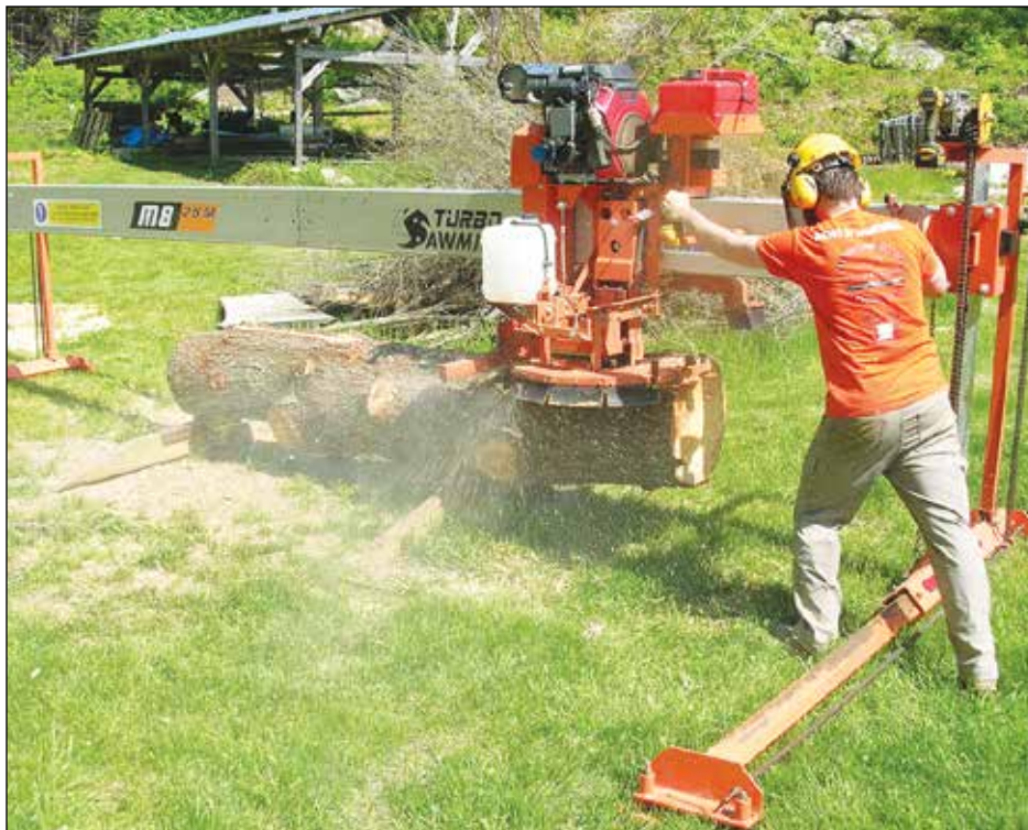
The Turbosawmill is fitted with a circular swing blade that allows for horizontal and vertical cuts. The mill can be set to accommodate whatever size of finished wood is desired. Photo by Faith Gillman
