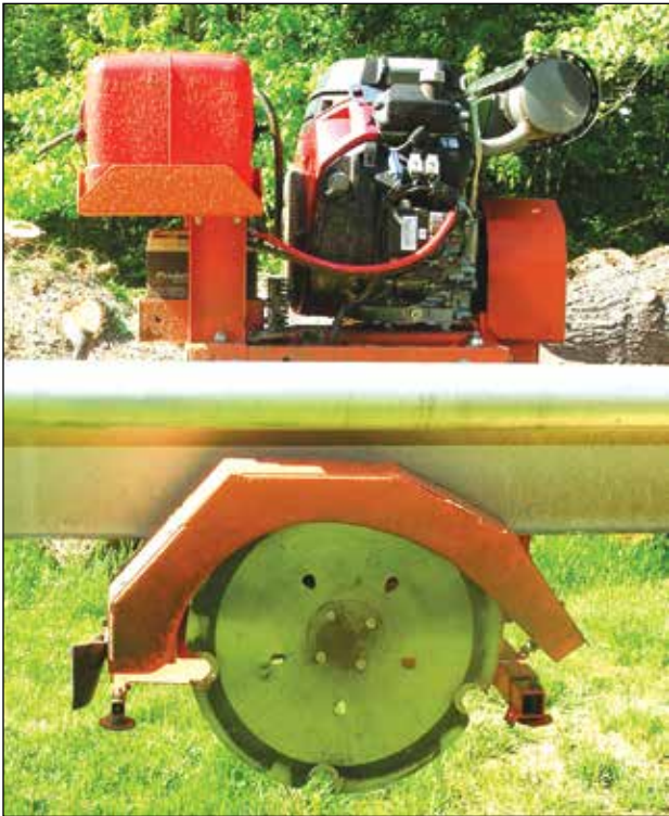
The huge blade of the sawmill has teeth inserts that can be sharpened or swapped out if damaged. Photo by Faith Gillman
